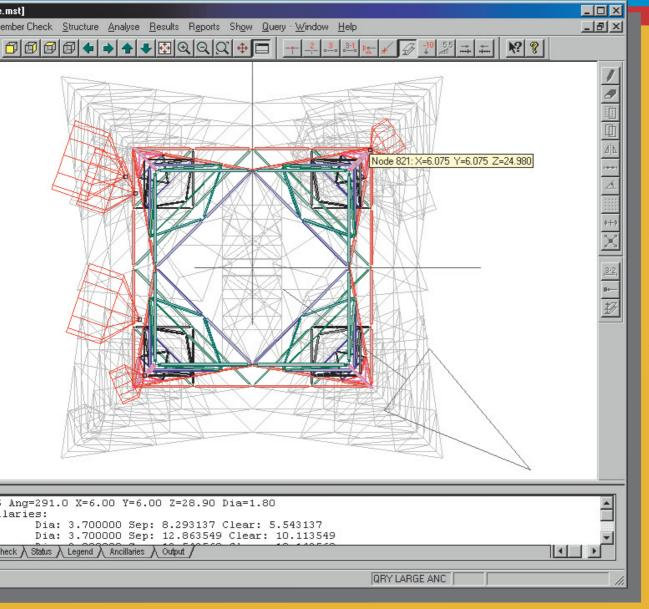
Automatic data checking detects a range of potential modelling problems in the tower geometry including overlaid and unconnected members.
