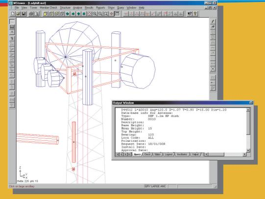
Member checking. Tower members can be checked automatically using member forces extracted directly from the analysis results. Member checks may be to:
